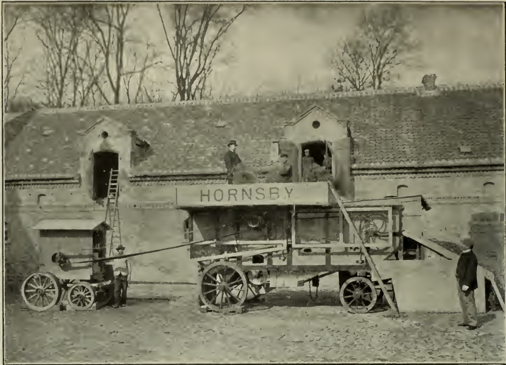
THRESHING MACHINE DRIVEN BY PORTABLE ELECTRIC MOTOR, AT CROTTORF.
